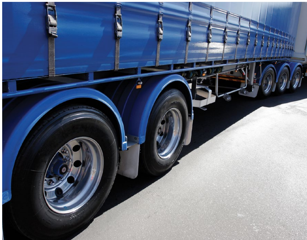
The B-triple represents a large upwards step-change in road freight productivity, carrying around twice the freight of a standard semi-trailer, while consuming in the order of seven per cent less fuel per tonne of freight than a B-double.
